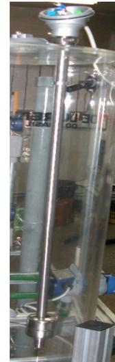
Figure 1 – Magnetic Float Level
