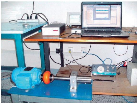
Figure 8 - Setup for bearing and related motor
