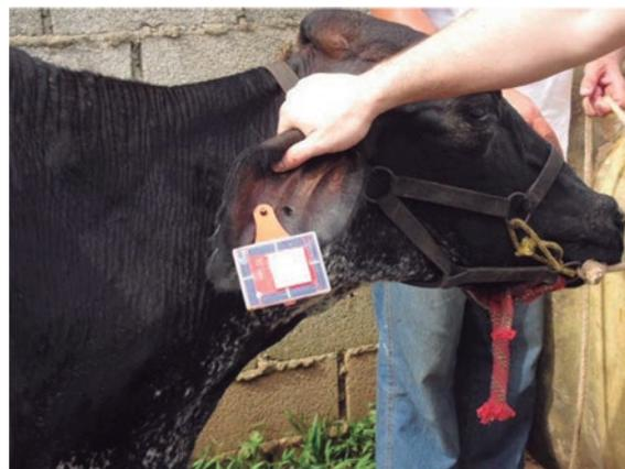
Figure 1 - Equipment installed in the left ear of the cow, comprised of a modem/transmitter, an antenna and a solar battery
