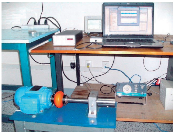
Figure 8 - Setup for bearing and related motor
