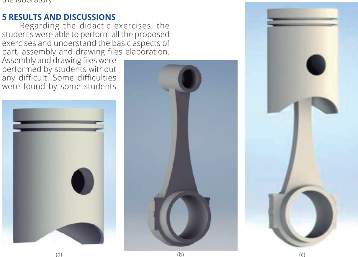
Figure 2 – Mechanism composed by the piston and connecting rod of an internal combustion engine. (a) Piston part. (b) Connecting rod part. (c) Complete mechanism assembly
